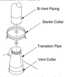
Figure 9 - Installing Transition Pipe and Starter Collar
